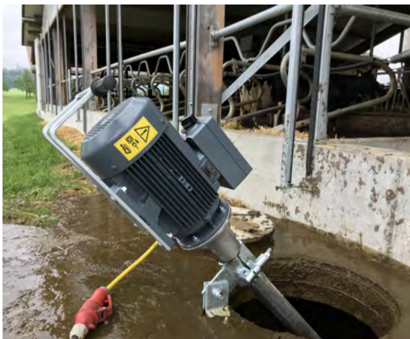
REKORDMIX - Closed tank with concrete top
